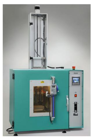
**The EB 16-II hot set tester** is made for hot set testing of cable material according to IEC 811-2-1. It is built on an ageing oven that performs well inside the apparatus requirements in IEC 811.
