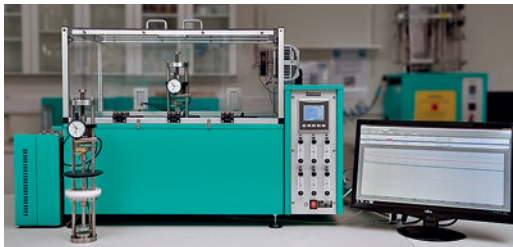
Stress relaxation test system for continuous testing of rubber in both tension and compression.
